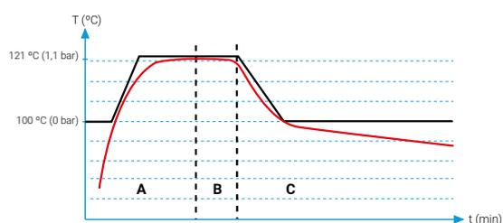
A = Calentamiento / Heating / Chauffage
