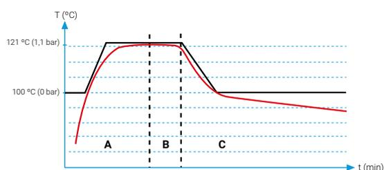
A = Calentamiento / Heating / Chauffage
